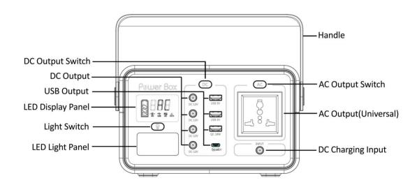
$^{\,\,\,\,\,\,\,\,\,}$ AC outlets, AC output voltage and frequency will vary according to different countries or areas. Please refer to the actual product before use. AC details are shown on the base of the unit.
